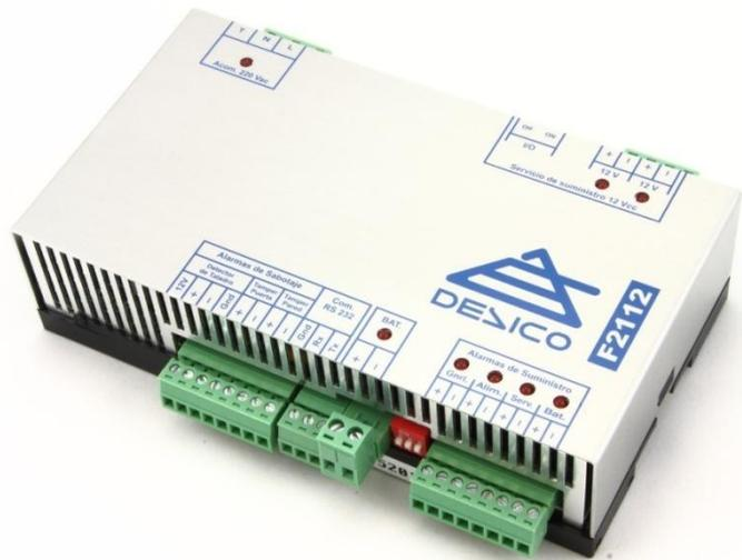
Through RS232 interface is possible to have remote monitoring of F2112 parameters, as output voltage for each output, current throughput for each output, and state of alarm signals.
